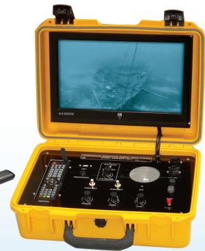
Working Status Display on LCD screen up to 18" TFT colour monitor, 12V DC power, variable LEDs light control, communication, and DVR with internal hard disk drive. Video data can be transferred to a standard USB flash drive.
